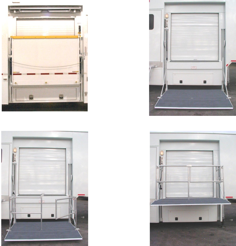
Figure 33: Platform Lift Progression
