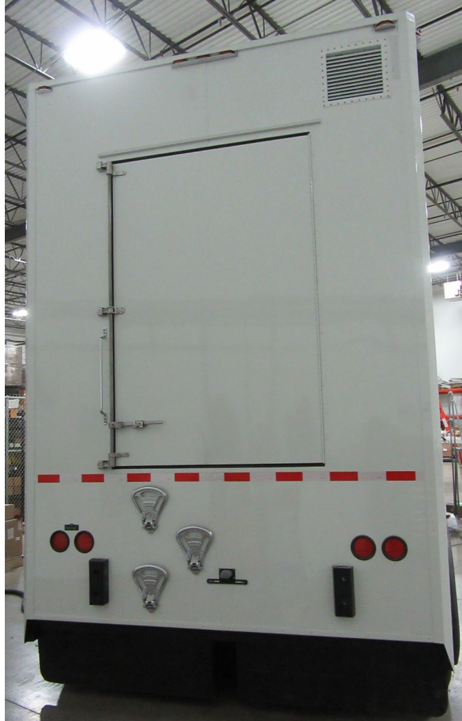
Figure 15: Magnet Room Helium Rear Door
