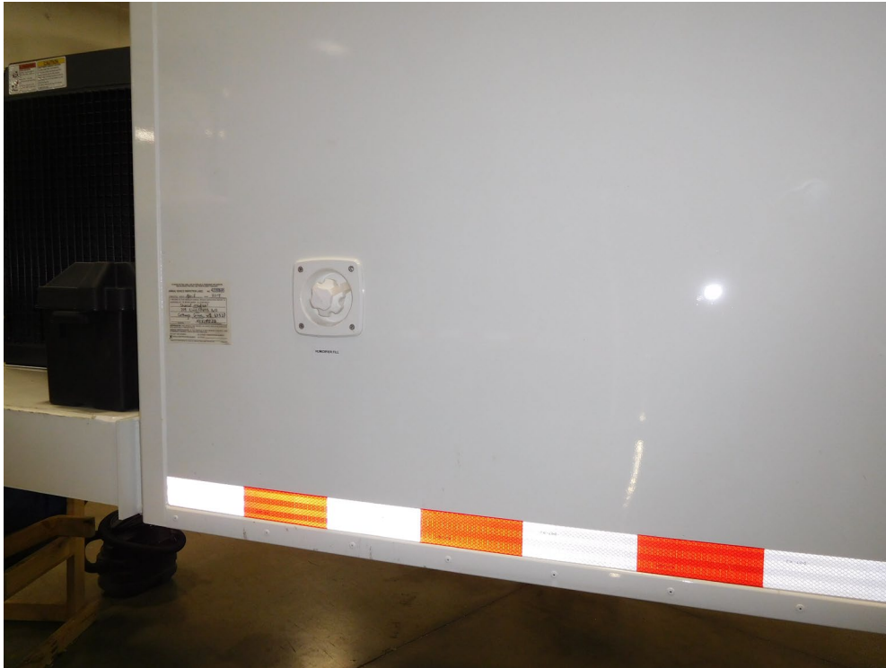
Figure 46: Humidifier External Water Connection
