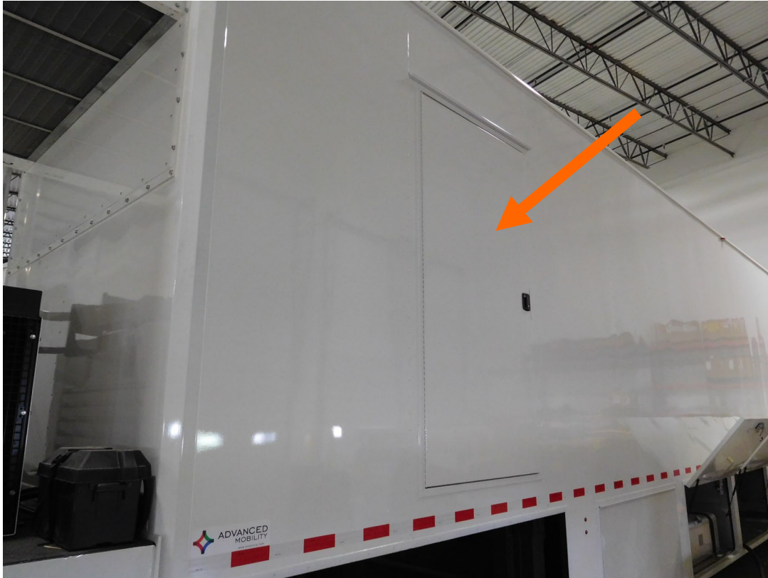
Figure 23: Emergency Exit / Service Door
