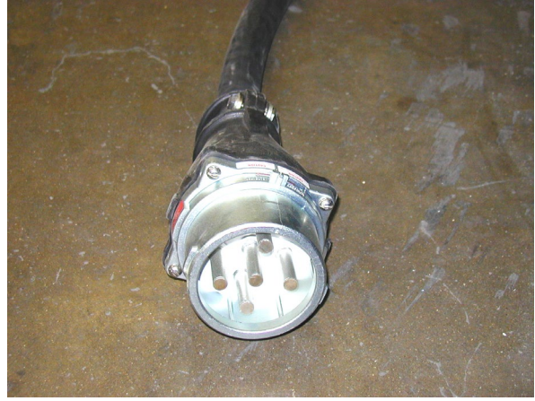
Figure 30: Shore Power Connection
