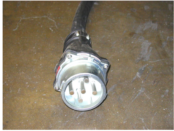
Figure 30: Shore Power Connection
