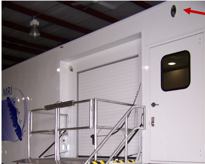
Figure 49: Entry Door Lighting
