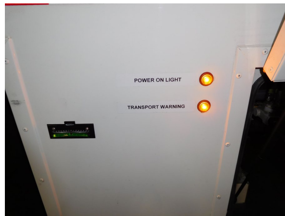
AC Power Light and Platform lift Transport Warning Light
