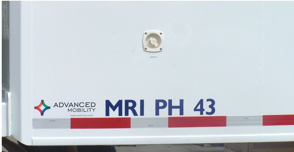
Figure 37: Humidifier External Fresh Water Connection
