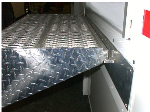
Figure 17: Stair Assembly (standard)
