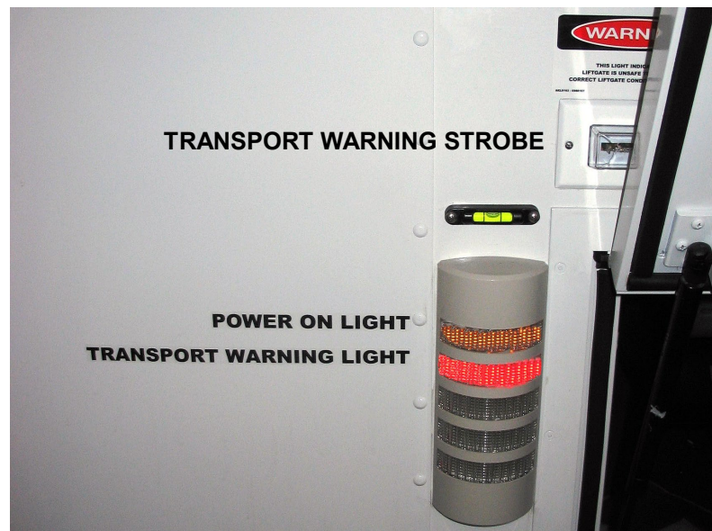
Figure 61: Lift Transport Warning Strobe
