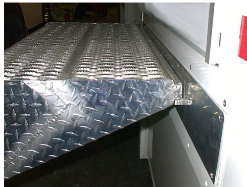
Figure 19: Stair Assembly (standard)
