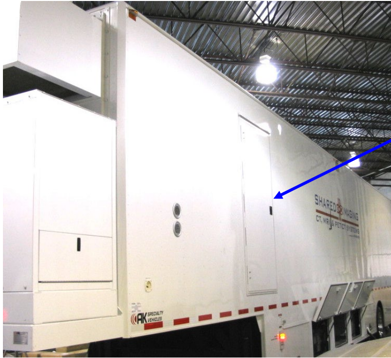
Figure 22: Emergency Exit / Service Door
