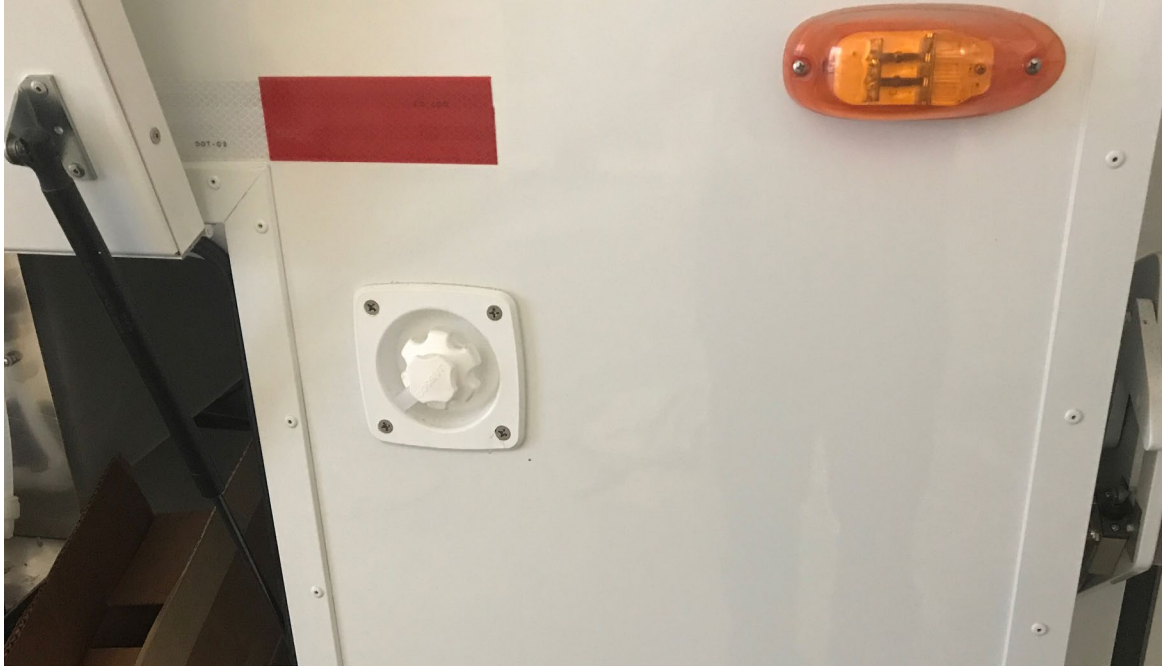
Figure 23: Humidifier Tank Fill
